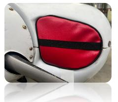
• **Preheating:** To maintain heat, install cowl plugs (carburetor and engine inlets) before preheating and after engine shutdown to maintain heat.
