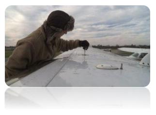
It's a common misconception that a thin layer of frost or ice is harmless, or that snow will blow off during takeoff. This can be a dangerous assumption. Contamination on wing and tail surfaces has contributed to numerous aircraft accidents.
